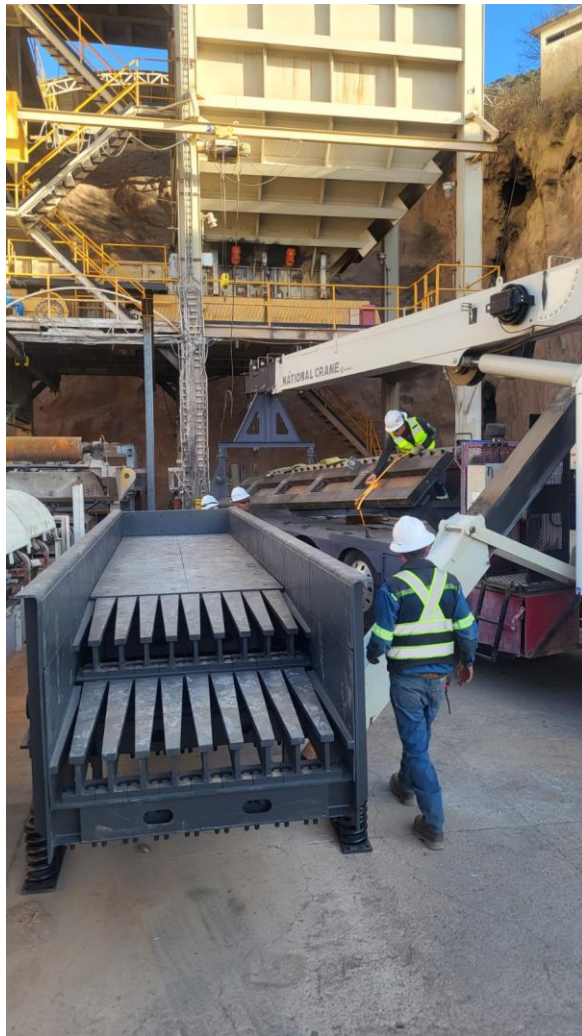
Figure 1: Grizzly vibrating screen delivered to site (left); leach tank rehabilitation (right)
