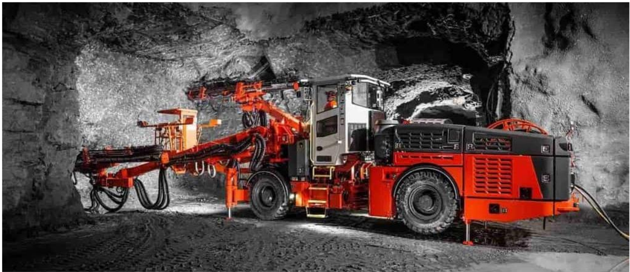
Figure 4 - Siton DW1-31 Longhole Production Drill (photo courtesy of Siton)
