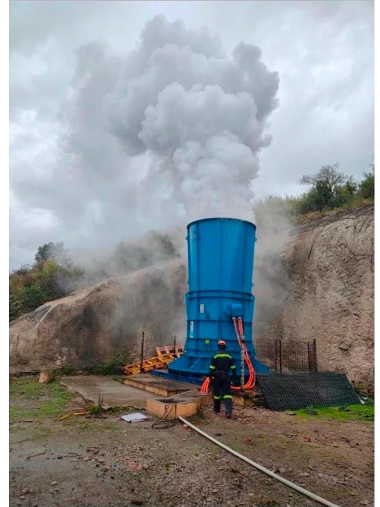
Howden ventilation fan removing exhaust air from underground
